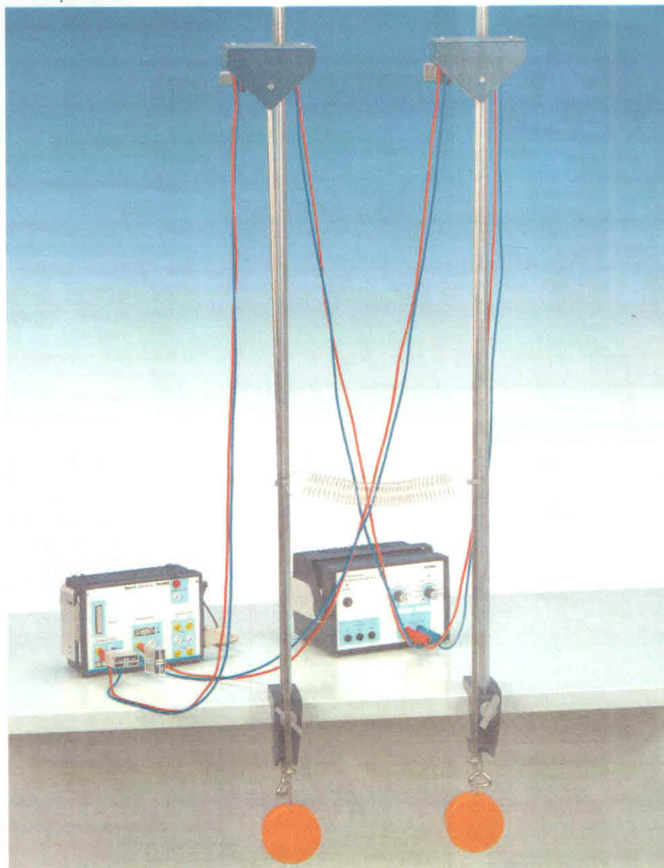
Fig. 1: Experimental set-up for the measurement of the vibrational period of coupled pendula.
